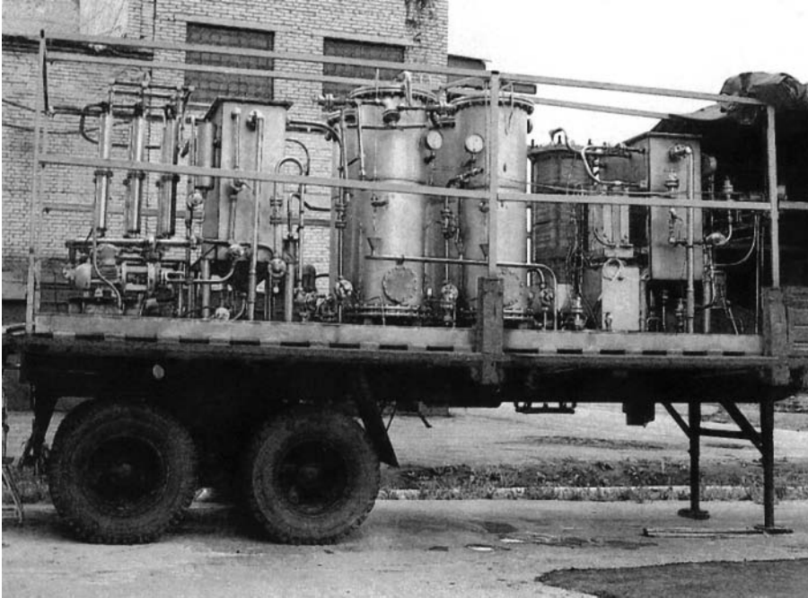
FIG. 24. The ECO-2 mobile system for LRW processing, containing ultrafiltration and electro dialysis equipment.
