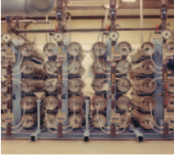
FIG. 20. A stationary hollow fibre reverse osmosis plant with a throughput of 60 m 3 /h.
